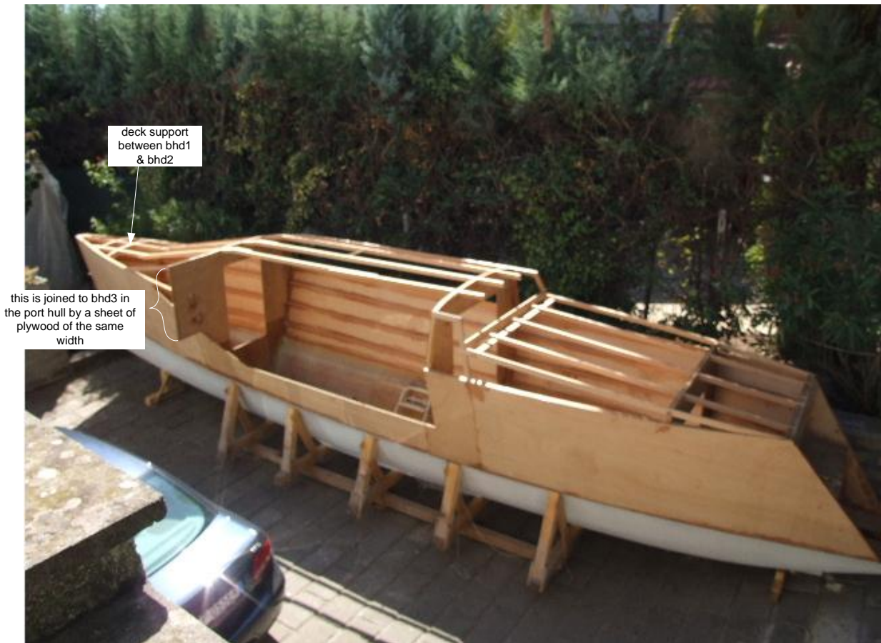
Figure 2: Starboard Hull After Adding Plywood Sheets
