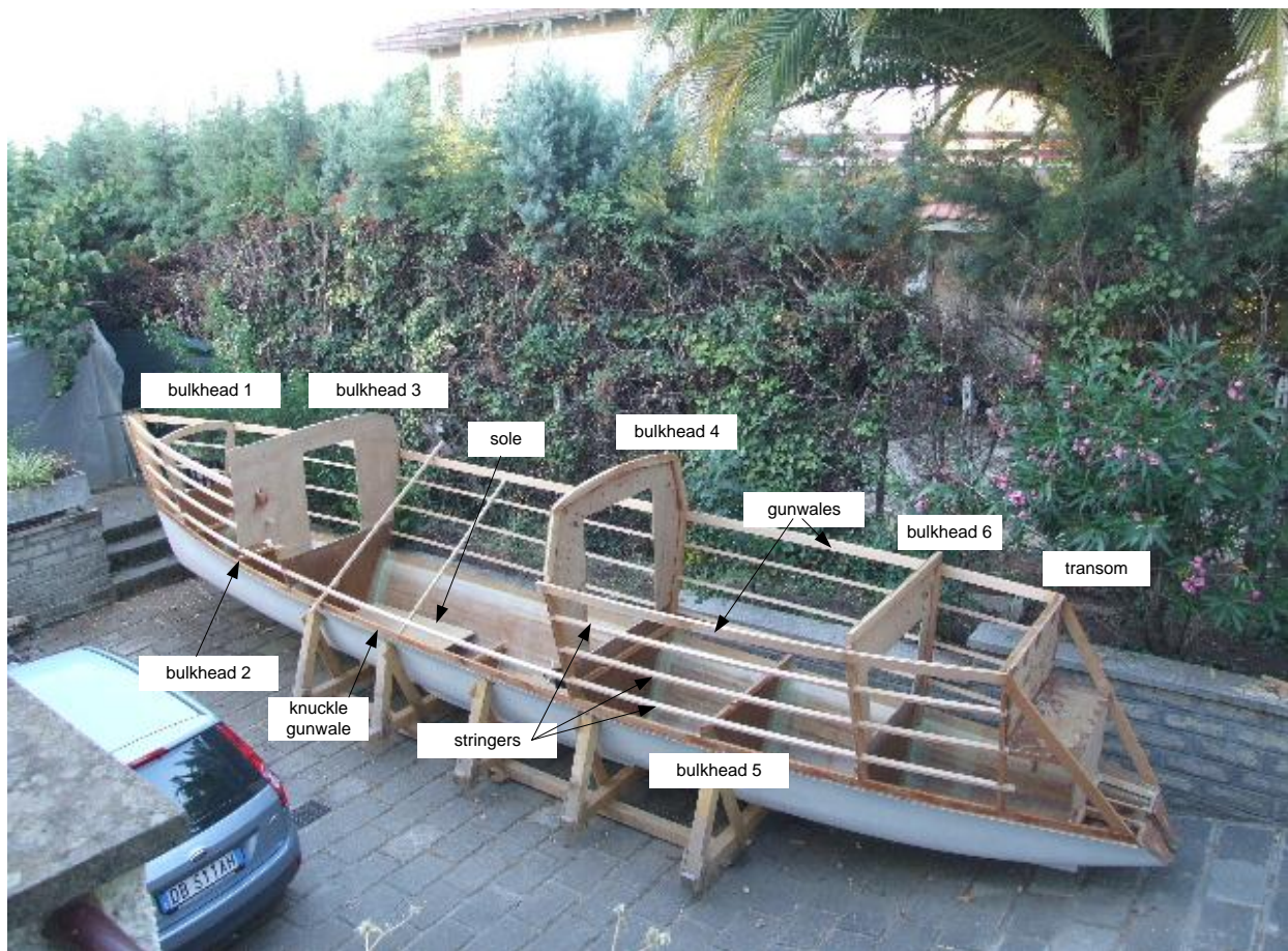
Figure 1: Starboard Hull Showing position of all Bulkheads and the Transom
